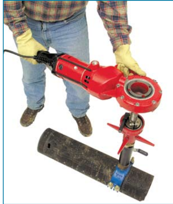
The Reed 700PD With The Optional TMPDA Adapter Fits 1 3 / 16 " Boring Bars
