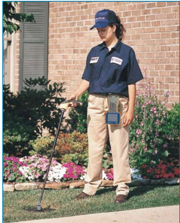
TouchRead® PitLid register and pit lid adaptor module being read with a PitProbe reading gun.
