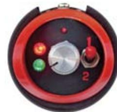
**Setting 1, Red LED:** The detector performs as a basic magnetic locator. All signals from ferrous metal objects, vertical or horizontal will be indicated with an Audio Tone and Red LED. No Green LED will show in setting 1
