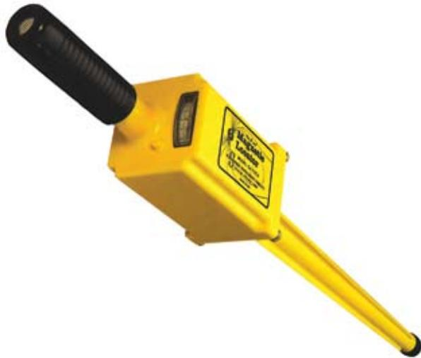
The GA-72CD Magnetic Locator detects the magnetic field of iron and steel objects. This locator is unique because it provides an audio signal and a visual indication of the signal strength and polarity. Although most objects can be located using either of the indications, simultaneous use of both will help you pinpoint an object, determine its orientation and identify magnetically detectable nonmetallic duct, cable and pipe.
