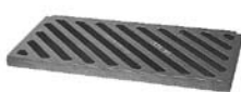
Type M5 Diagonal Bar Grate Approx. 225 sq. in. of Opening, 1 1/4" Wide Openings Between Bars, Not Suitable for Bicycle Traffic
