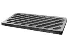
Type M3 Diagonal Bar Grate Approx. 315 sq. in. of opening, 2 1/8" Wide Opening Between Bars, Not Suitable for Bicycle Traffic
