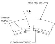
Figure 1 Starter shim and wedge arrangement for 14", 18", and 20" sizes.
