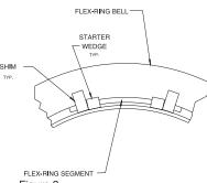
Figure 2 Shim and wedge arrangement for 16", 24", 30", 42", 48", and 54" sizes.
