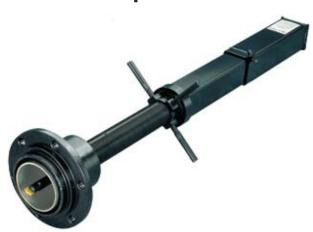
The TapMate<sup>™</sup> Drilling Machine is an affordable, lightweight machine for drilling 3" thru 12" sizes. Used with a tapping sleeve, it can cut PVC, A/C, Ductile Iron, Cast Iron and Steel pipe.
