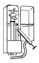
Standard utility bilge pump attaches to vent tube to remove water from waterway, insuring a clean sample in the future, and preventing freezing.
