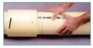
Tear-Down — Nylon spline is pulled out and pipes pulled apart. Use silicone lubricant (available through your local Team EJP sales office) if pipe is to be disassembled.
