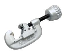
These copper tubing cutters have a large grip knob for comfort during use. Reamer is built inside grip knob for convenience and safety. Wide rollers yield a square cut while thin cutter wheel profile insures a quick, clean cut.
