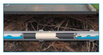
The Ultimate Resin: Our patented resin provides the strength and flexibility to permanently repair any cracks and voids. The resin is able to cure in the presence of water and eliminates the possibility of being washed away.
