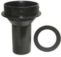
This reduced neck valve box riser is specifically designed to be used in valve boxes that have previously had a riser installed. Minimum height gained is approximately 2". The top flange securely holds the extension in the pavement. When used with the dirt shield, it becomes a conventional slide riser for standard use.
