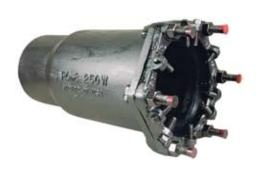
The MJ Cut-In Sleeve used with the Resilient Wedge Cut-In Valve offers a simple quick method for installing additional gate valves in existing lines.
