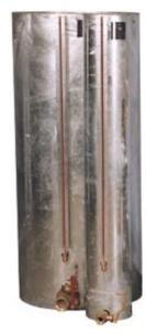
Pictured above are 10 gallon and 100 gallon tanks, ordinarily used together as are the one cubic foot and ten cubic foot tanks. In nearly all cases two tanks are recommended, the smaller for low and intermediate tests and the larger for high flow tests.
