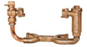
The Meter Setter/Resetter is designed to easily retrofit existing meter installations to include a dual check backflow preventer. This is accomplished without the high risk of cutting into old service piping, or the expensive process of digging up and replacing existing meter boxes or pits.
