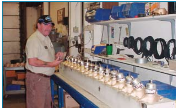
Refurbished meters getting new registers, chambers and gaskets
