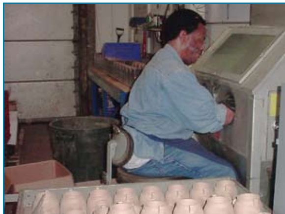
Old brass main cases are sandblasted and painted as part of the refurbishing process.
