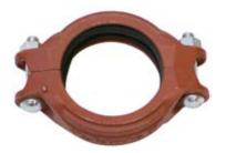
Style 31 Couplings are designed to provide a strong component for ductile iron pipe systems of AWWA dimensions. The Style 31 FlushSeal<sup>®</sup> gasket is specifically designed for ductile pipe surfaces and provides an efficient triple seal. Rigid radius grooved ductile iron systems with Style 31 couplings are comparable with flanged ductile iron systems.
