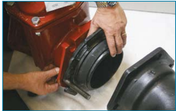
Align and Insert Bolts From Valve Side
