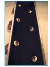
This cutaway view of the inside of a tapped Ductile Iron pipe clearly shows that the corporation stops do not damage the cement-mortar lining of the pipe.
