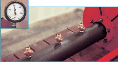
DIPRA's direct tapping tests were conducted on 4-foot Ductile Iron pipe specimens 6 inches in diameter. Tests involved three <sup>3</sup>/<sub>4</sub>-inch taps on one specimen and three 1-inch taps on the other specimen as shown here. The initial internal water pressure of 70 psi was gradually increased to 1,000 psi (inset photo) in an attempt to cause failure.
