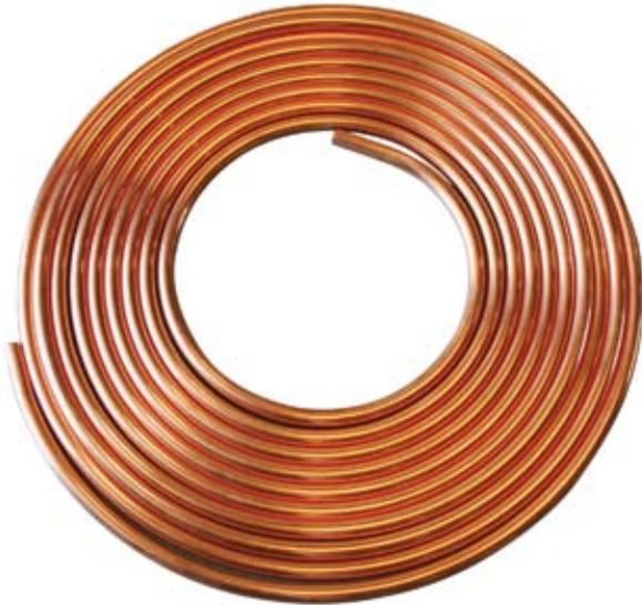
Type K, soft copper tubing, remains free from rusting and is highly resistant to corrosion and scale formation. Type K has a heavy wall thickness for underground services from the water main to the house connection. It is conductive to enable thawing and its flexibility allows it to conform to underground trenching.
