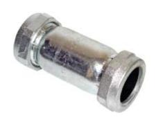
No pipe threading—No working to exact measurement—No special tools. Pipe is not weakened by thread cutting. Simply stab on the coupling, center over pipe ends and tighten with a wrench. It's quick, easy, permanent!
