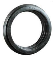
Concrete Manhole Adapters (CMA) help eliminate leaks around pipe entering manhole walls, yet are flexible enough to permit lateral pipe movement without destroying seal integrity. It is particularly useful for pipe to which concrete will not adhere, such as plastic pipe.
