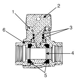
Ball Valves are ideal for use in water service lines. Tightness in both directions at all pressures, easy turning, non-binding, and minimum pressure loss—these characteristics are added to good engineering design, quality material and precise manufacturing.
