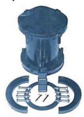
The 5¼" B-62-B hydrant is extended at the barrel flange above the ground line, eliminating any need for excavation. The B-62-B Top Extension Kit includes all parts necessary to extend the hydrant.
