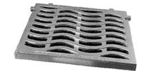
Type M3 Sinusoidal Grate Approx. 170 sq. in. of opening, Grate has break-off section so that curb back can be added when curb is installed
